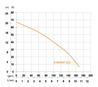
Shaft Speed: 3450 rpm Outlet: 80mm, 3in
